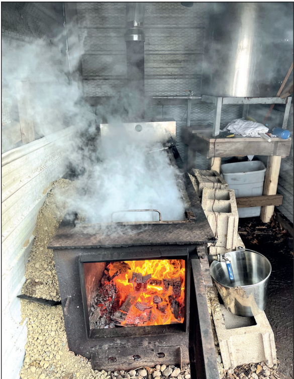
Peterson’s sugar shack is a literal hotbed of activity during maple syrup season. The storage tank that holds sap overnight is in the upper right; it cooks down in the silver trough that’s sitting atop the fire, then is run into the silver pail at the lower right after the majority of the water cooks off. Peterson carries the pail into his garage for some of the final steps.
