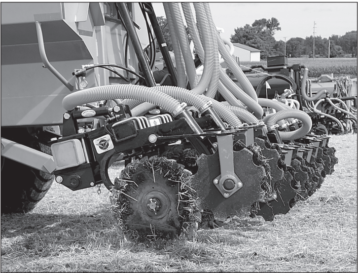
Staff photo by Jake Nelson In order to fertilize their fields, farmers employ the use of a small machine known as the manure injection system.
